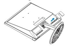
4. Lose four screws to remove the column.
