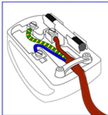
1. The GREEN AND YELLOW wire must be connected to the terminal in the plug which is marked with the letter "E" or by the Earth symbol
