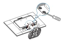
3. Remove the screws from hinge cover.
