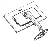
2. Loosen the assembly screws, then detach the neck from the display.
