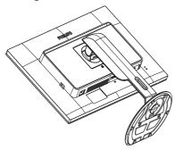
While keeping the release button pressed, tilt the base and slide it out.
