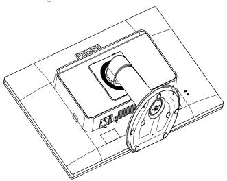
2. Remove the screws from hinge cover.
