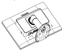
2. Remove the screws from hinge cover.
