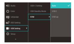
If you would like to use a DP and/or HDMI cord to input into your device, use the USB-C and USB-B ports with the USB cord being in direction USB upstream.
