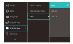
If you would like to use a DP and/or HDMI cord to input into your device, use the USB-C1 and USB-C2 ports with the USB cord being in direction USB upstream.
