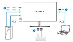
Enter to OSD menu. Go to KVM layer and select "Auto", "USB C" or "USB Up" to switch the control of peripherals from one device to another. Simply repeat this step for switching the control system using one set of peripheral.
