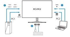
3. Enter to OSD menu. Go to KVM layer and select "Auto", "USB C" or "USB Up" to switch the control of peripherals from one device to another. Simply repeat this step for switching the control system using one set of peripheral.
