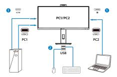
Enter to OSD menu. Go to KVM layer and select "Auto", "USB C1" or "USB C2" to switch the control of peripherals from one device to another. Simply repeat this step for switching the control system using one set of peripheral.
