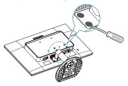
3. Remove the screws from hinge cover.
