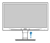
Place the monitor face down on a smooth surface, taking care to avoid scratching or damaging the screen. Then lift the monitor stand.
