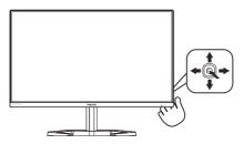
To access the OSD menu on this Philips display simply use the single toggle button on the rear side of the display. The single button operates like a joystick. To move the cursor, simply toggle the button in four directions. Press the button to select desired option.
