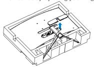
Use a screwdriver to remove the screws on the arm, and then detach the arm/stand from the monitor.
