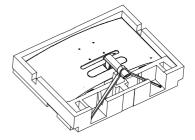
2. Remove the hinge cover from monitor body by using your fingers.
