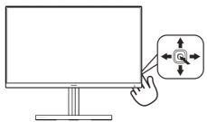
To access the OSD menu on this Philips display simply use the single toggle button on the backside of the display bezel. The single button operates like a joystick. To move the cursor, simply toggle the button in four directions. Press the button to select desired option.
