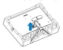
Use a screwdriver to remove the screws on the arm, and then detach the arm/stand from the monitor.
