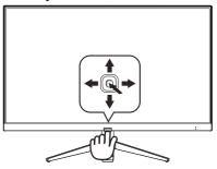
To access the OSD menu on this Philips Display simply use the single toggle button at the bottom of the Display bezel. The single button operates like a joystick. To move the cursor, simply toggle the button in four directions. Press the button to select desired option.
