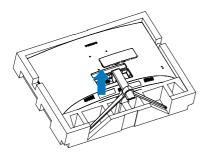
Use a screwdriver to remove the screws on the arm, and then detach the arm/stand from the monitor.
