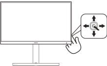
To access the OSD menu on this Philips display simply use the single toggle button on the rear side of the display. The single button operates like a joystick. To move the cursor, simply toggle the button in four directions. Press the button to select desired option.
