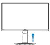
2. Place the monitor face down on a smooth surface. Pay attention not to scratch or damage the screen. Then lift the monitor base.
