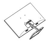
Use your fingers to loosen the screw located at the bottom of the base,and remove the base from the stand.
