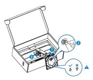
Note Secure the arrow of the base towards the front and fix to the column tightly.
