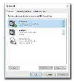
To change the sound output source, right click on the audio default device, click "Disable" then, it will switch to the next sound output device, if you want to switch it back, right click on the source, click "Enable"
