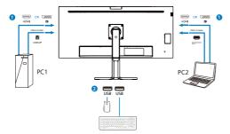
3. Enter the On-Screen Display (OSD) menu. Go to the KVM tab and select "Thunderbolt", or "USB UP" to switch the monitor view from one device to another. To switch to another monitor view, simply repeat this step.
