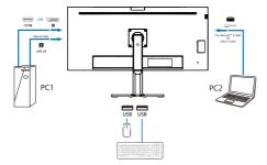
2. Enter the On-Screen Display (OSD) menu. Go to the KVM tab and select "Auto", "Thunderbolt", or "USB UP" to switch the monitor view from one device to another. To switch to another monitor view, simply repeat this step.
