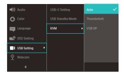
If you would like to use a DP and/or HDMI cord to input into your device, use the Thunderbolt input  $\square / ^{(90W)}$  and USB UP ports with the USB cord being in direction USB upstream.
