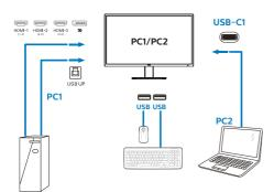
Enter to OSD menu. Go to KVM layer and select "Auto", "USB-C1" or "USB up" to switch the control of peripherals from one device to another. Simply repeat this step for switching the control system using one set of peripheral.
