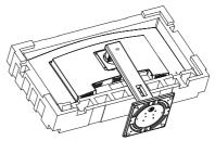
2. While keeping the release button pressed, tilt the base and slide it out.
