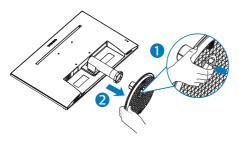
3. Press the release button to detach the base column.
