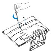
Move the stand into position as shown in picture. Then use a screwdriver to remove the screws, and then detach the stand from the monitor.
