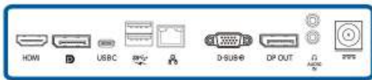
I/O back panel connector diagram
