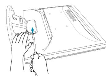
2) Remove the 4 screws and then remove the base from the LCD monitor.
