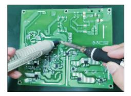
S19-5 Lift the bulk cap. up and away from the PCB.
