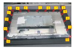
S11 Disconnect the panel lamp from the connectors of the panel and interface board and then put it aside. Disconnect the LED cable from the connector of the interface board, then release the LED cable by tearing off the 2pcs tapes.
