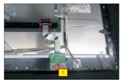
Use a Philips-head screwdriver to remove 15(13+2)pcs screws for unlocking the middle bezel. (No.1~13 screw size=M3x5, Torque=5±0.5kgfxcm No.14~15 screw size=M2x3.3, Torque=0.8~1.2kgfxcm)
