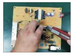
S19-4 Take out bulk cap. pin solder with soldering iron and absorber.
