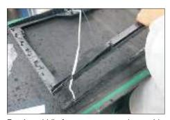
Put the middle frame on a protective cushion, then tear off 2pcs mylar, then tear off the 2pcs aluminum foil and 2pcs rubber pads. Use a Philips-head screwdriver to remove 2pcs screws for unlocking the left and right Mic boards.
