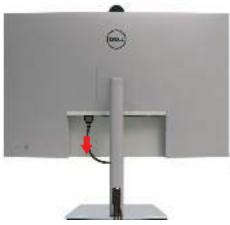
Remove stand from the product.(Press the stand release button, lift the stand up and away from the monitor)
