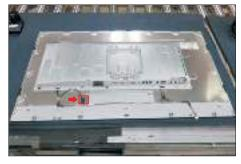
S19 Take away the bracket chassis module and then put the bracket chassis module on a protective cushion.
