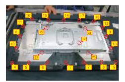
Tear off the tape on the back of the LED cable, then disconnect the panel lamp cable and touch FFC cable from the connectors, and then remove the conductive foam from the middle frame.
