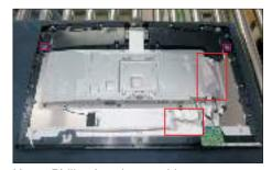
Use a Philips-head screwdriver to remove 2pcs screw for unlocking the USB board, and disconnect the two USB FFC cables from the connectors of the board, then release the USB board from the hooks of the middle frame. Tear off 1pcs aluminum foil for unfixing the touch FFC wire, and then disconnect LED wire from the connector of the board.
