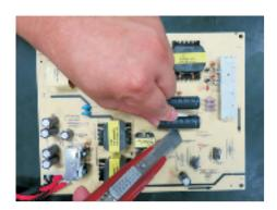
S23-3 Cut into the bottom of bulk cap. and pullit up carefully.
