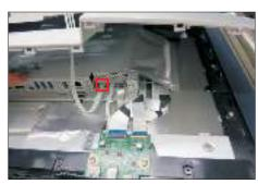
Use a Philips-head screwdriver to remove 2pcs
