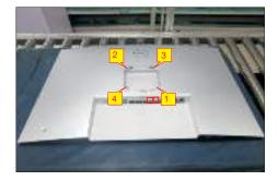
Tear off screen protector, then wedge your fingers between rear cover and the middle bezel on the corners of the top side of the monitor to release the rear cover, then use one hand to press the middle bezel, the other hand to pull up the rear cover in order of arrow preference for unlocking the rear cover.
