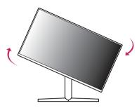
4 Complete the installation by rotating the monitor 90° as shown below.
