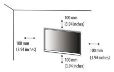
To install the monitor to a wall, attach a wall mounting bracket (optional) to the back of the monitor. Make sure that the wall mounting bracket is securely fixed to the monitor and to the wall.
