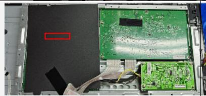
Remove the screws on the mainboard and power board
