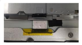
S14 Disassemble LVDS cable from Panel
