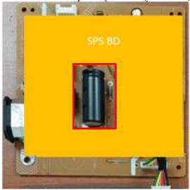
S22-1 Cut the glue between bulk cap. and PCB with a knife
