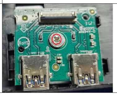
Remove the screw on the usb board
