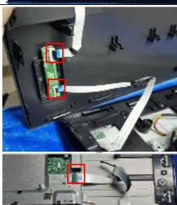
open the cover on the keyboard/ usb board and then pull out the cables
