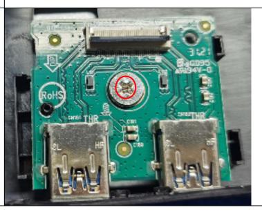
Remove the screw on the usb board
