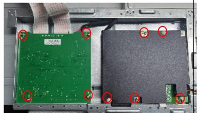
Remove the screws on the mainboard and power board
