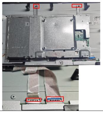
Remove the two screws on the mainframe and then disconnect the FFC cables
