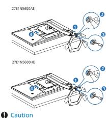
Place the monitor face down on a smooth surface. Pay attention not to scrath or damage the screen.
