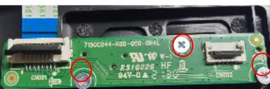
Remove the 3pcs screws on the keyboard
