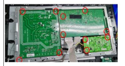
Remove the screws on the mainboard and power board
