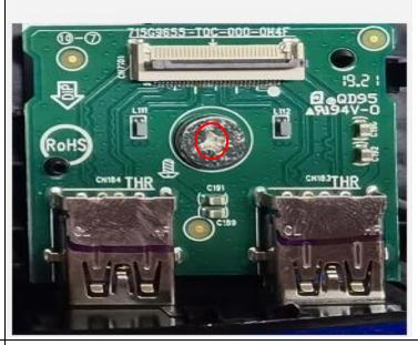
Remove the screw on the usb board
