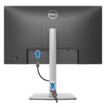
3. Connect the DisplayPort, HDMI, USB-C (C-C), or USB-C (C-A) cable from your monitor to the computer.
