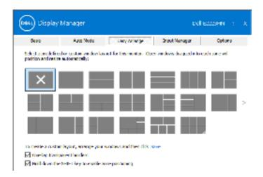
If you are using multiple monitors in an array or matrix, **Easy Arrange** layout can be applied across to all the monitors as one desktop. Select "**Span multiple monitors**" to enable this feature. You need to align your monitors properly to use it effectively.
