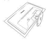
2. Press the locking clips to detach the base stand away from the base column.
