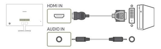
The audio function is not supported if the source device is connected using the HDMI-DVI cable.
