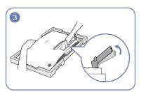
While holding the monitor, lift the stand neck in the direction of the arrow and adjust it, as shown in the image.
