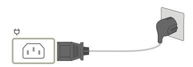
To use the product, connect the power cable to a power outlet and the  ${\pmb \nabla}$  port on the product.
