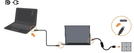
2) Connect Type-C power adapter to the left or right side of L15 and connect L15 to the mobile phone with a USB-C cable.
