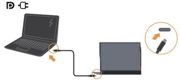
2) Connect the USB-C port of mobile phone and L15 with a USB type-C cable. (Electronically marked cable, current rating: 5A).
