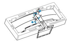
3. After attaching the base, erect the monitor with both hands on holding the monitor together with styrofoam firmly. Now you can pull out the styrofoam. Notice this monitor is curved design, when you pull out styrofoam, do not squeeze the panel to avoid broken panel.
