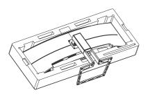
2. Loosen the assembly screws, then detach the neck from the display.
