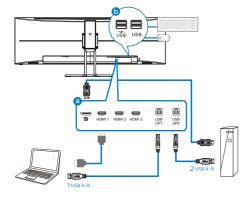
Enter to OSD menu. Go to KVM layer and select "USB up1" or "USB up2" to switch the control of peripherals from one device to another. Simply repeat this step for switching the control system using one set of peripheral.
