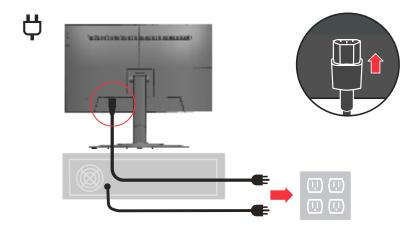
6. Connect the cables with cable clip.
