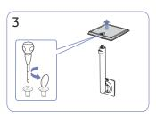
Unfasten the connecting screw at the bottom of the stand base, and then remove the stand neck from the stand base by pulling it in the arrow direction, as shown in the figure.
