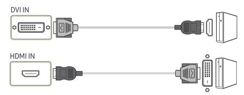
The audio function is not supported if the source device is connected using the HDMI-DVI cable.
