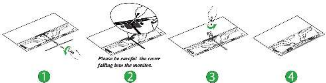
Figure.1. Installing and Removing the Base
