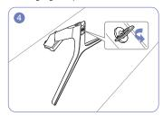
Remove the stand neck from the stand base by turning the screw in the arrow direction as shown in the figure.
