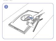
Press the lower part of the monitor with one hand, and pull the stand with the other hand in the direction of the arrow as shown in the figure.
